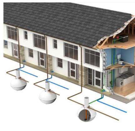
Photograph 48 - Example of Rainwater Harvesting
