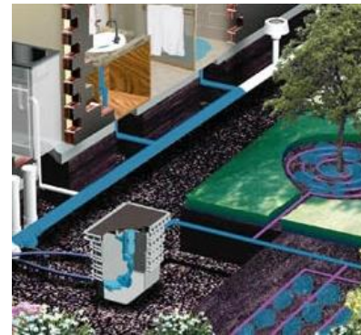
Photograph 49 - Example of Grey Water Recycling
